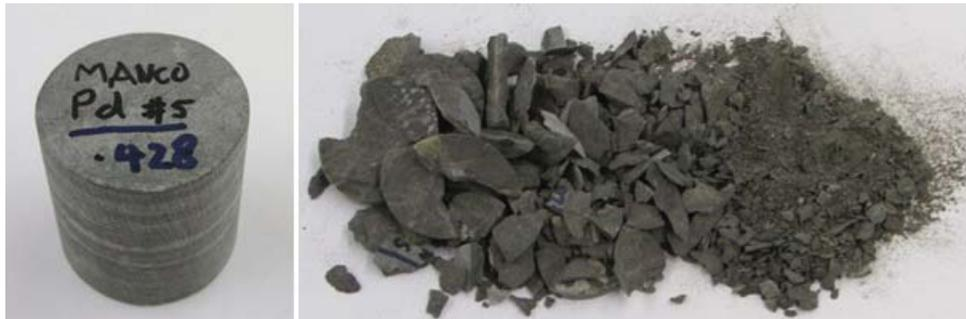
Fig. 9. A Mancos outcrop shale plug before (left) and after microwaving (right).
