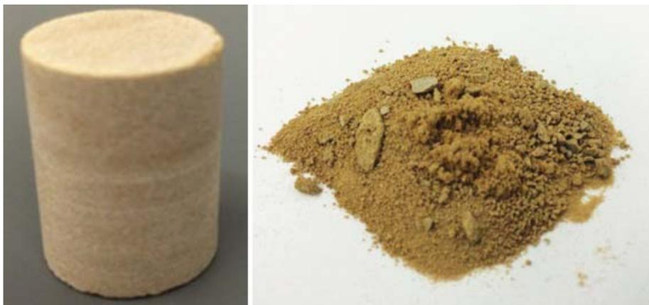
Fig. 6. Tight Tennessee sandstone before and after microwaving. 20.1 seconds microwaving completely obliterates the rock plug.
