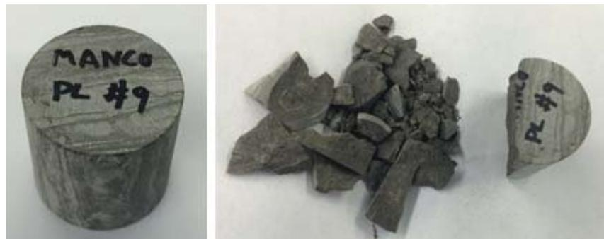
Fig. 10. A Mancos outcrop shale plug before (left) and after microwaving (right).
