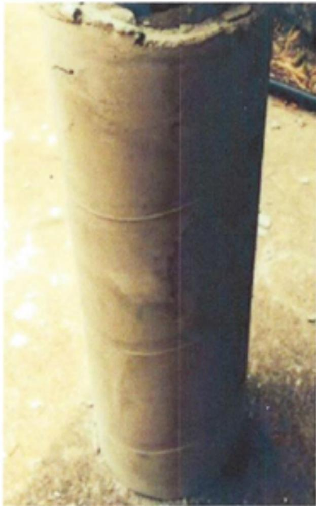
Simulated blocked perforated casing target before pulsing
