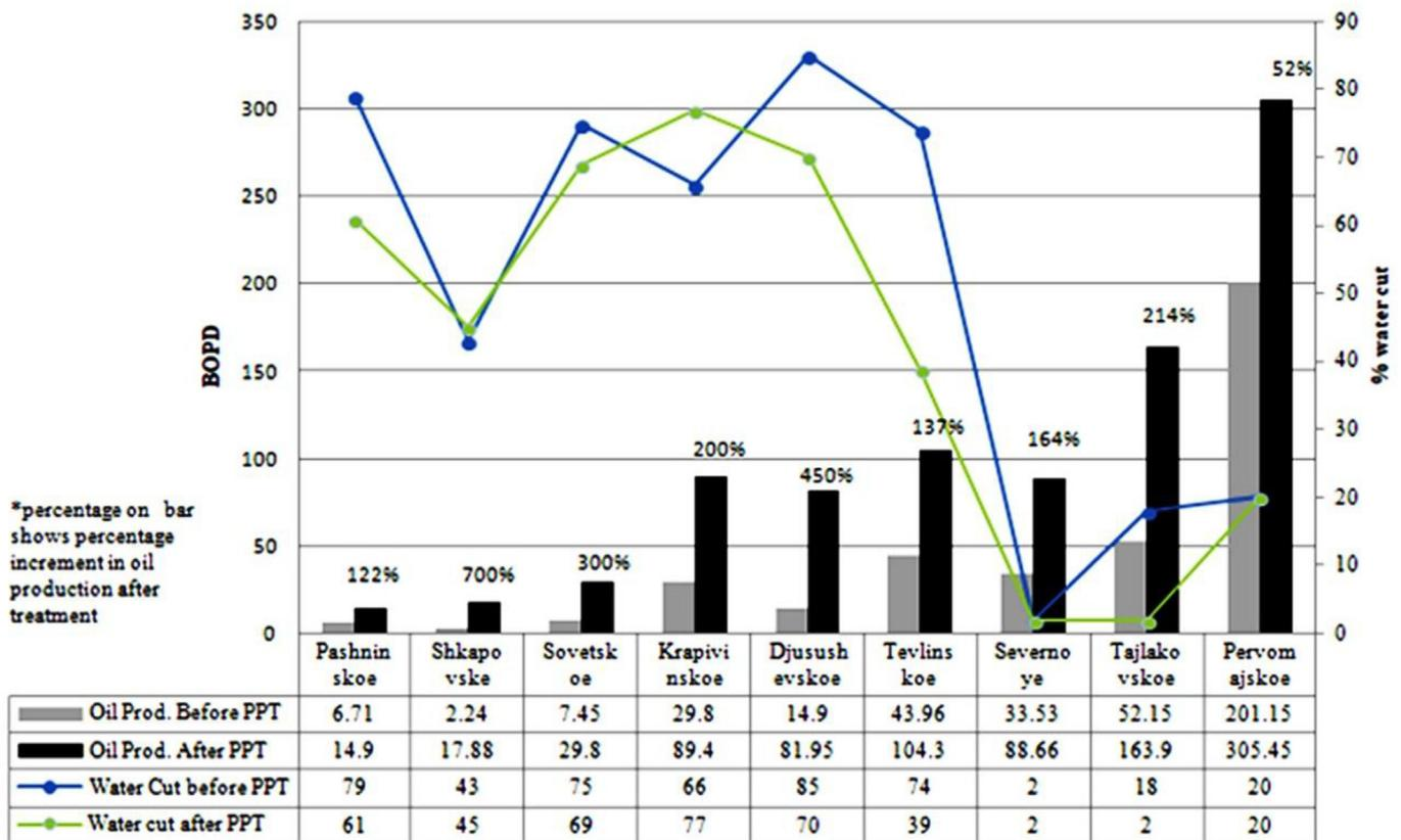
Fig. 7. Oil production and % water cut before and after of PPT treatment on production well of few oil fields of Russia (data from Novas Energy, 2015).<sup>2</sup>
