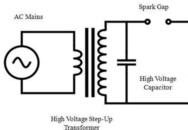
Fig. 5. Simple electric circuit diagram showing formation of plasma arc across spark plug.
