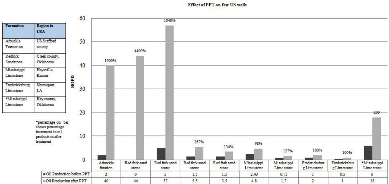
Fig. 8. Effect of PPT on oil production from sandstone and limestone formations of few US fields.<sup>4</sup>
