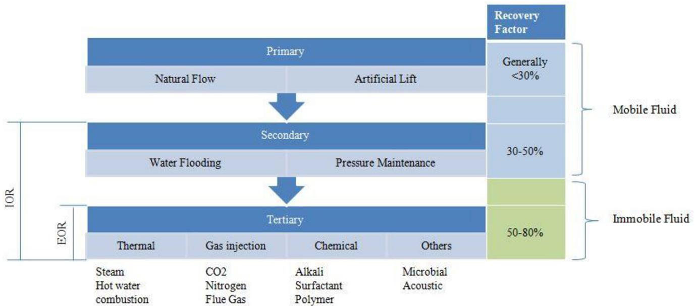
Fig. 1. Defining improved oil recovery (IOR) and enhanced oil recovery (EOR) (Stosur et al., 2003).
