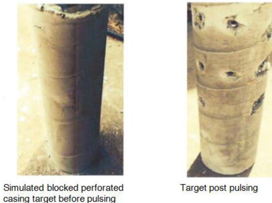
Fig. 4. Effect of PPT on the cement integrity after and before its application.<sup>1</sup>
