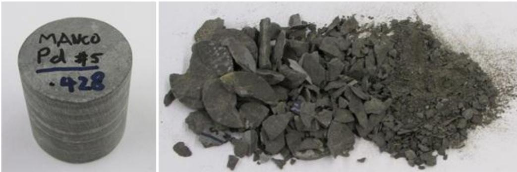
Fig. 10. Mancos outcrop shale plug before (left) and after microwaving (right).
