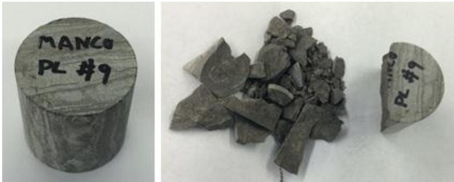
Fig. 11. Mancos outcrop shale plug before (left) and after microwaving (right). Half of the plug was intact after microwaving.
