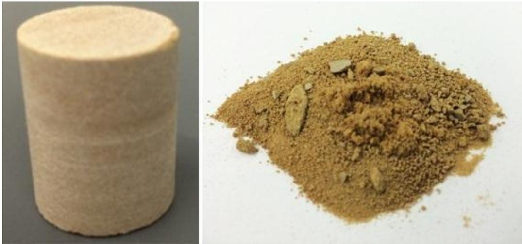
Fig. 7. Tight Tennessee sandstone before and after microwaving. 20.1 seconds microwaving completely obliterated the rock plug.
